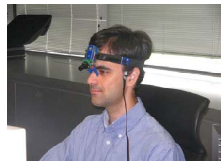
The Jazz-novo recording the human behaviour during decision-taking processes by one of the OTS-operators.
